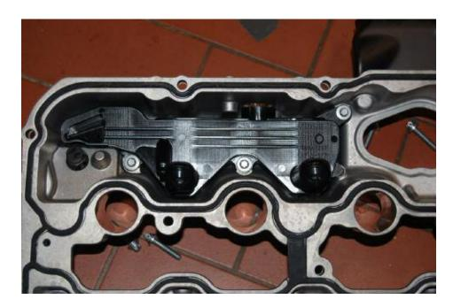
Note: If the exhaust system produces blue smoke, it is necessary to check whether the engine is also drawing oil into the combustion chamber through the crankcase breather, which suggest that there is a fault in the area of the crankcase breather. A clear sign of a problem is an oiled up clean-air pipe.
