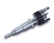
This injector design permits injection pressures of up to 200 bar and extremely quick opening of the nozzle needle. In this way, it is possible to inject fuel into the combustion chamber under conditions released from the power cycles limited by the valve opening times.
