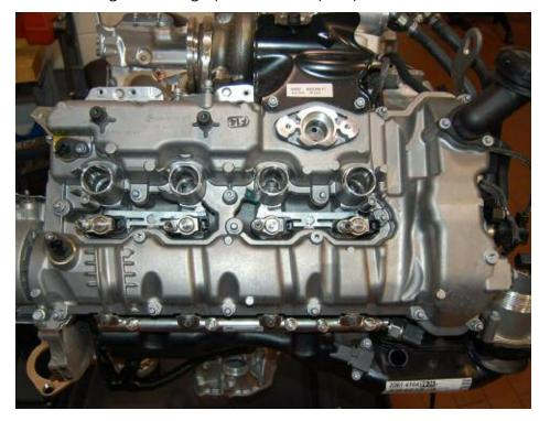
Cyclone separators are contained within the cylinder head covers as removable plastic components. There are no crankcase ventilation valves on the N63 engine, but there are externally mounted check valves similar to the N54.
