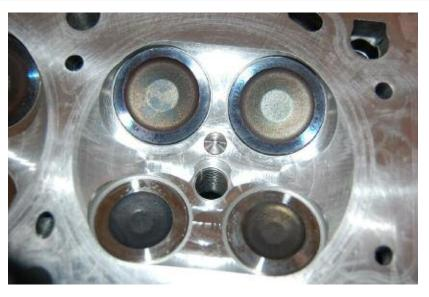
The intake port features a trailing edge for creating more intensive charge movement. The fuel injectors and spark plugs are arranged transversely adjacent to each other in the center of the combustion chamber roof.
